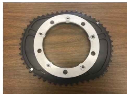
Figure 1. Custom inner chainring affixed to the rear of the Osymetric chainring. Bolt holes are spaced 36° apart.
