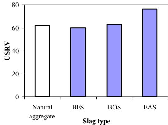
Figure 10. Slip/skid resistance of paving blocks containing coarse and fine slag simultaneously
