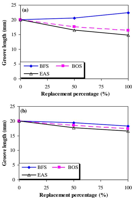
Figure 7. Groove length of paving blocks containing, (a) Coarse slag and (b) Fine slag
