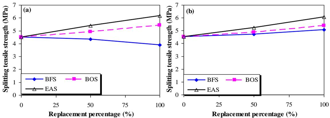
Figure 5. Tensile splitting strength of paving blocks containing, (a) Coarse slag and (b) Fine slag
