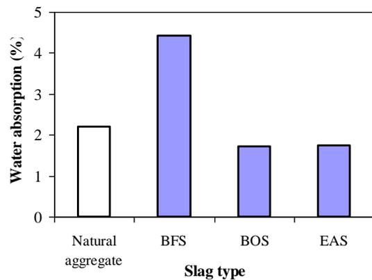
Figure 12. Water absorption of paving blocks containing coarse and fine slag simultaneously
