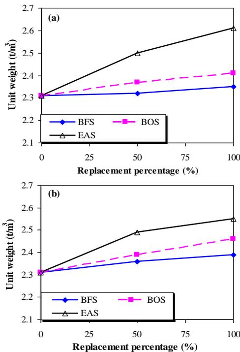
Figure 2. Unit weight of paving blocks containing, (a) Coarse slag and (b) Fine slag
