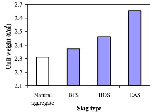
Figure 3. Unit weight of paving blocks containing coarse and fine slag simultaneously
