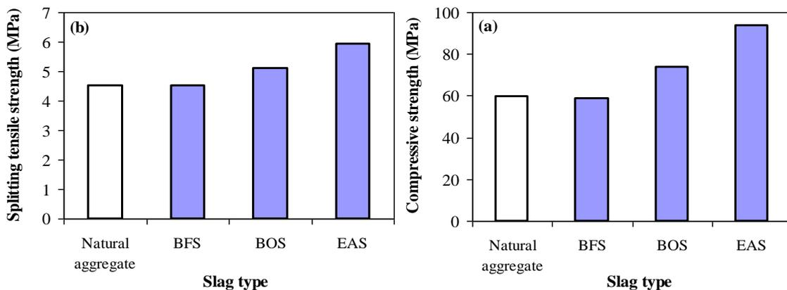
Figure 6. Strengths of paving blocks containing coarse and fine slag simultaneously, (a) Compressive strength and (b) Tensile splitting strength
