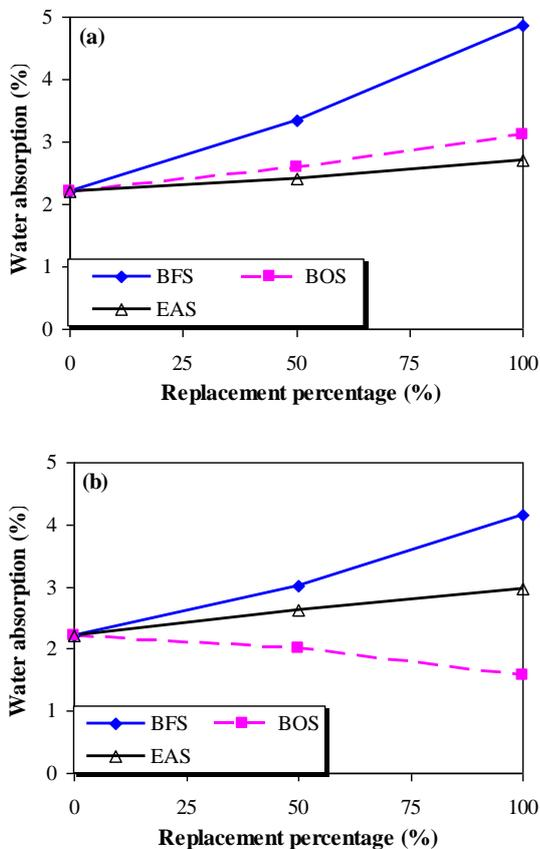
Figure 11. Water absorption of paving blocks containing, (a) Coarse slag and (b) Fine slag
