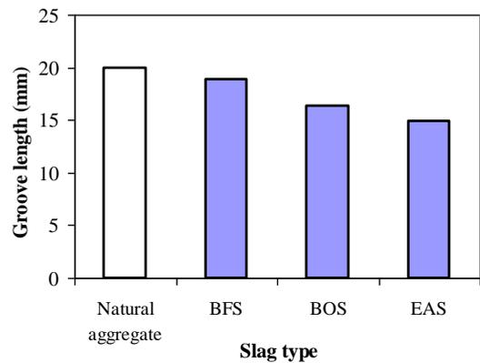
Figure 8. Groove length of paving blocks containing coarse and fine slag simultaneously
