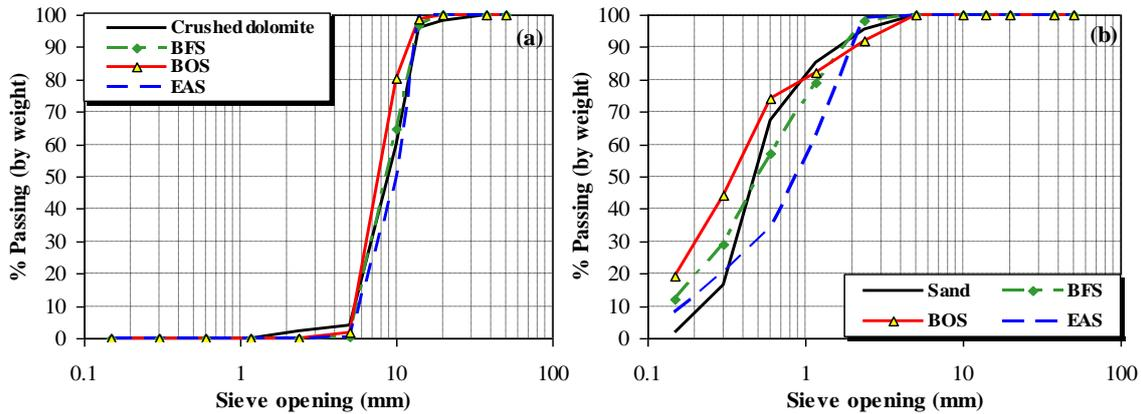
Figure 1. Sieve analysis of aggregates, (a) Coarse aggregate and (b) Fine aggregate
