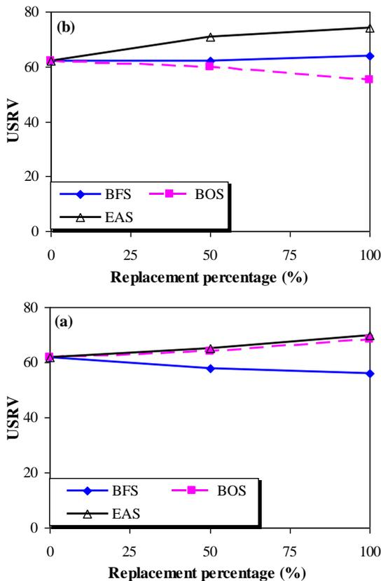
Figure 9. Slip/skid resistance of paving blocks containing, (a) Coarse slag and (b) Fine slag
