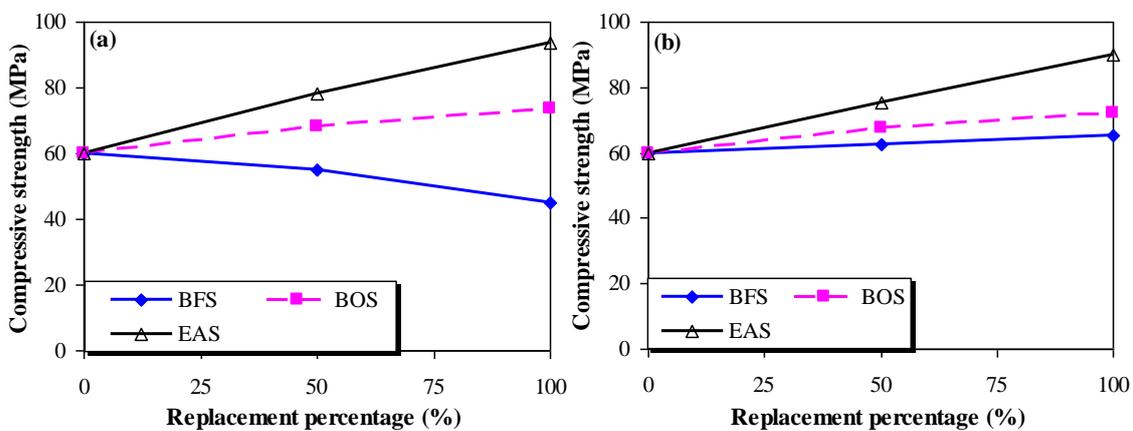
Figure 4. Compressive strength of paving blocks containing, (a) Coarse slag and (b) Fine slag
