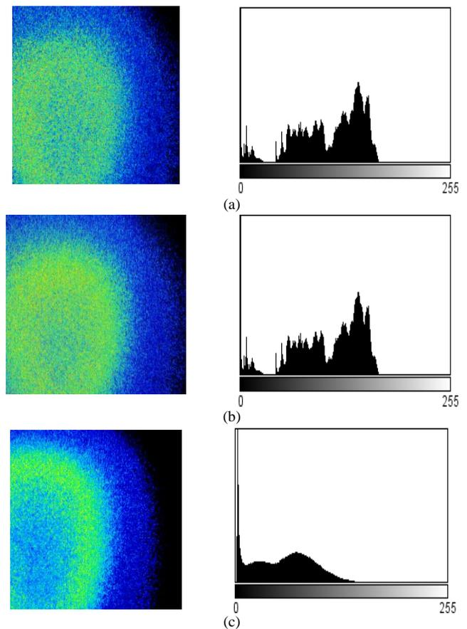
Figure 4. a) Bioactivity map and histogram of corn grains harvested at 4 km/h, b) Bioactivity map and histogram of corn grains harvested at 6 km/h, c) Bioactivity map and histogram of corn grains harvested at 8 km/h.
