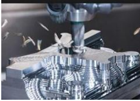
Figure 2. Raw material steel (H13/SK61) removed by cutting tools in CNC machine
