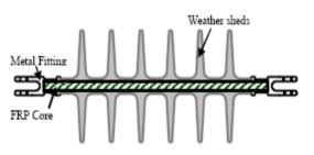
Figure 1: The SIR insulator structure with fibreglass insulator bars FRP
