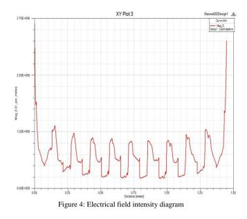
It is clear from this figures the electric field intensity is more than the normal value so the probability of electrical break in polluted condition is more than the condition without pollution.
