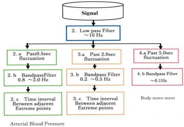
Figure 4. Sensor systems of signal processing flow.
