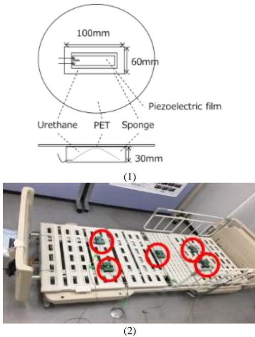
Figure 3. Piezoelectric vibration sensors and bed sensor installation positions.
