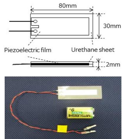
Figure 1. Piezoelectric pillow sensor.
