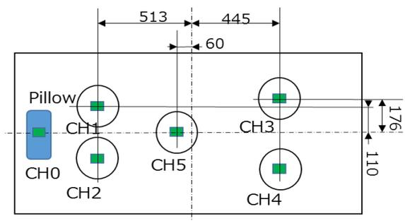
Figure 5. Layout of piezoelectric load sensor positions.
