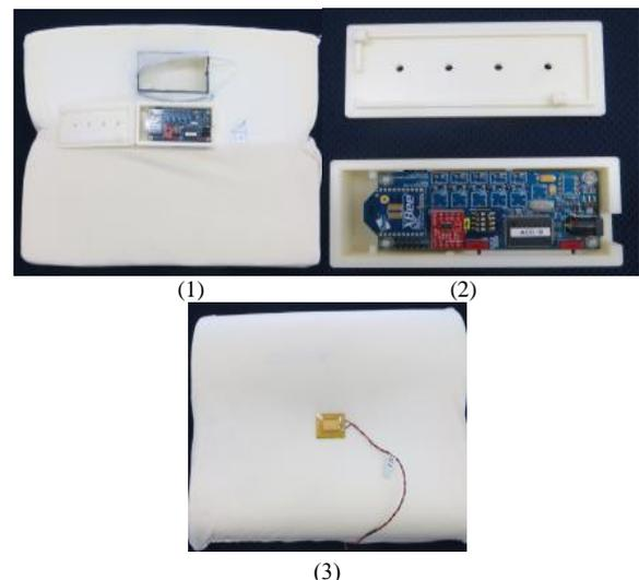
Figure 2. Pillow sensor and radio systems
