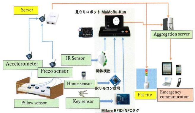
Figure 8. New monitoring system for quality of life.
