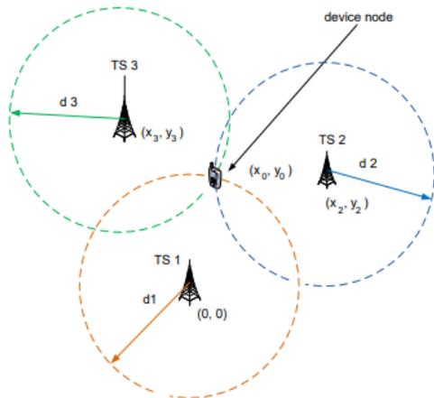
Figure 1. Illustration of the TOA method
