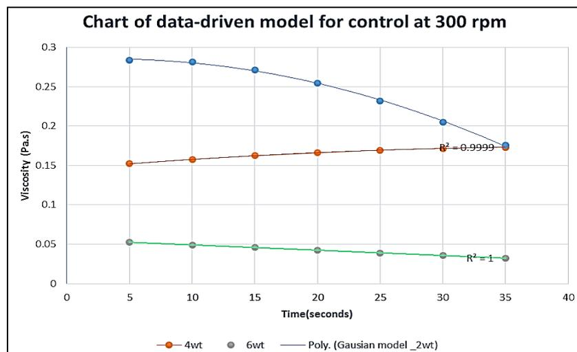
Figure 6. Chart of data-driven model for 2wt, 4wt and 6wt. %  $\text{Na}_2\text{CO}_3$  at 300 rpm
