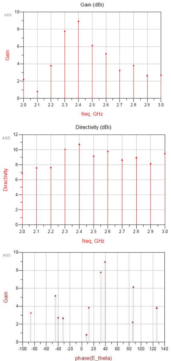
Figure 11. Gain, Directivity and Gain vs Phase (E-Theta)
