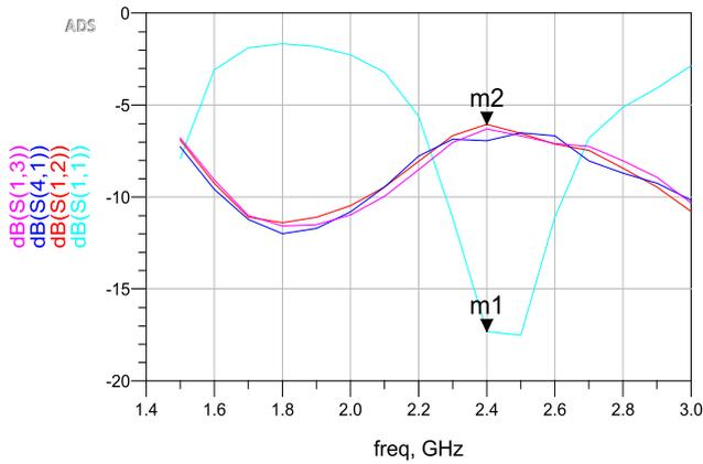
Figure 8. Results of designed 2-way Wilkinson Power Divider
