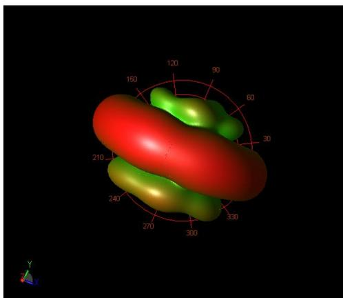
Figure 10. 3D Radiation pattern of 1x4 array antenna
