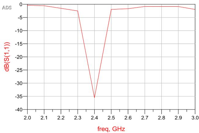
Figure 9. Return loss for 4-element array antenna
