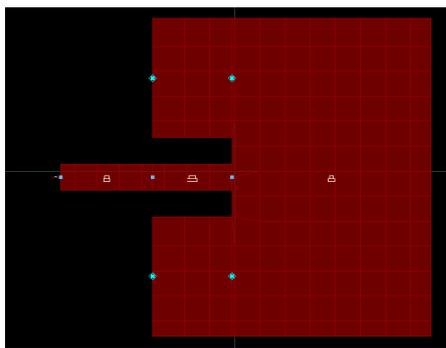
Figure 2. Designed Inset fed Microstrip patch antenna
