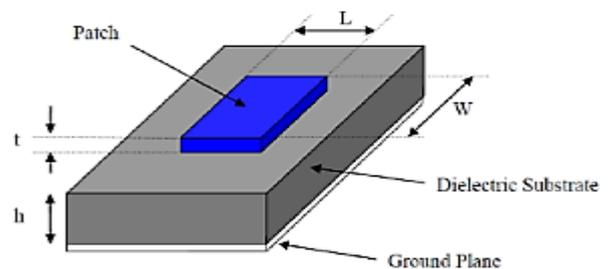
Figure 1. Structure of microstrip patch antenna[1]
