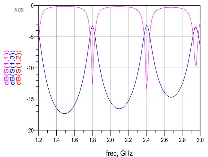
Figure 7. Results of designed 4-way Wilkinson Power Divider
