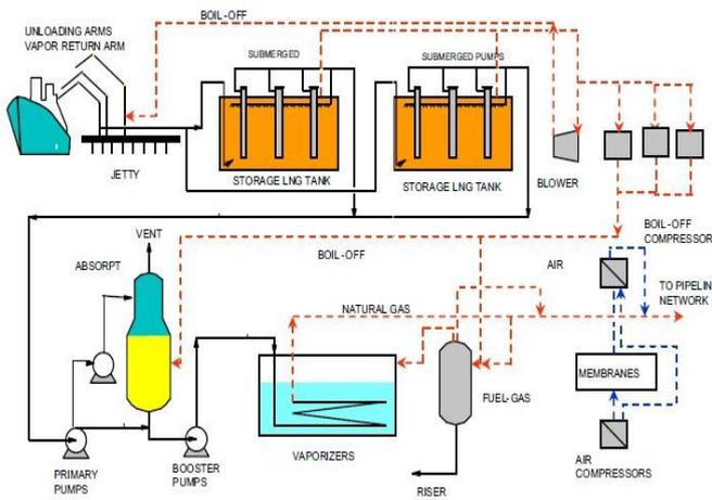
Figure 1. Typical onshore LNG terminal operation [2]
