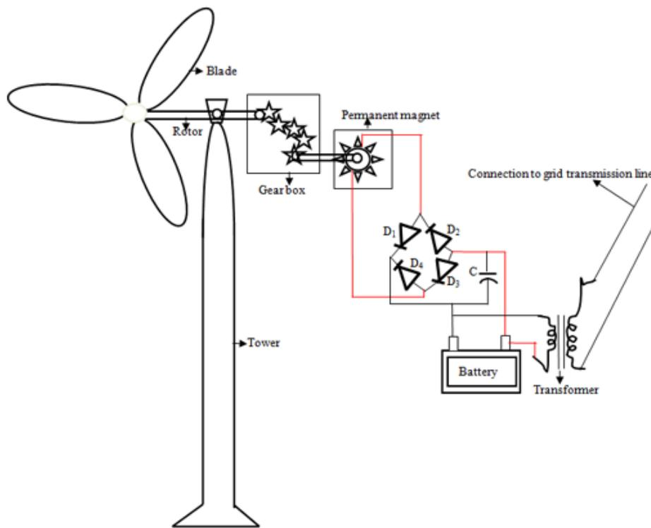
Figure 1. Wind energy conversion components
