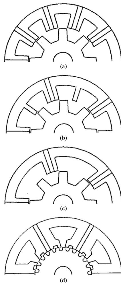
Figure 2. a) Traditional structure, b) E-core structure, c) C-core structure, d) Multi-tooth structure
