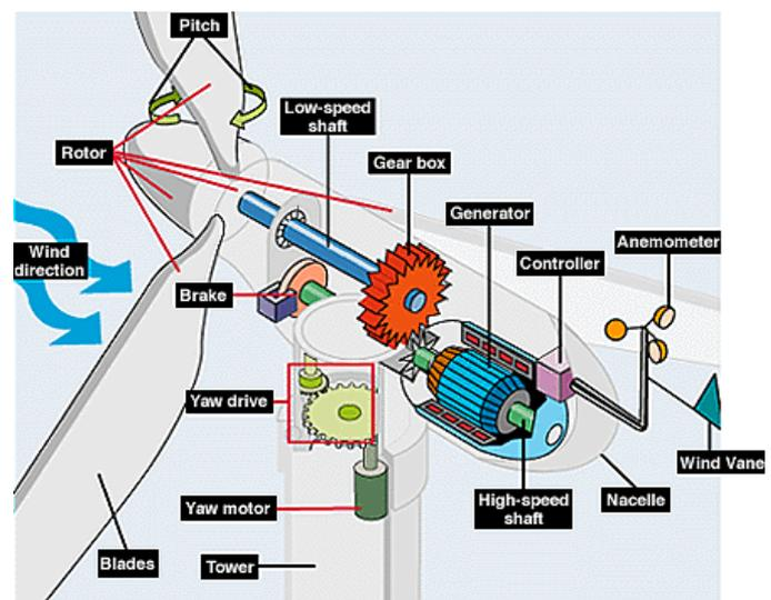
Figure 1. Components of a conventional horizontal-axis wind turbine (Saad & Asmuin, 2014)
