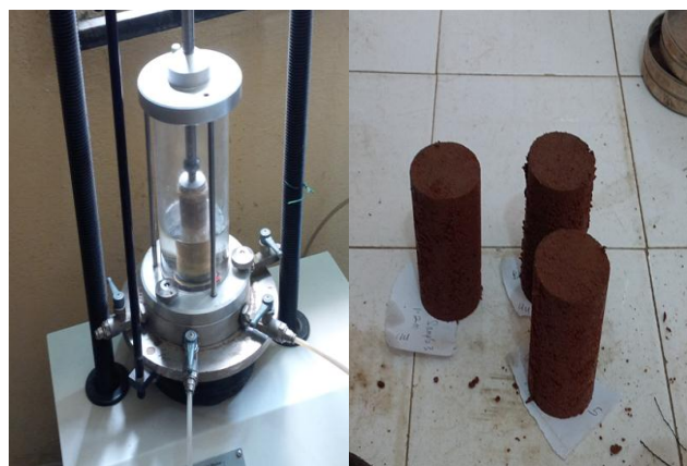
Figure 1. Triaxial process and prepared soil sample for the triaxial test
