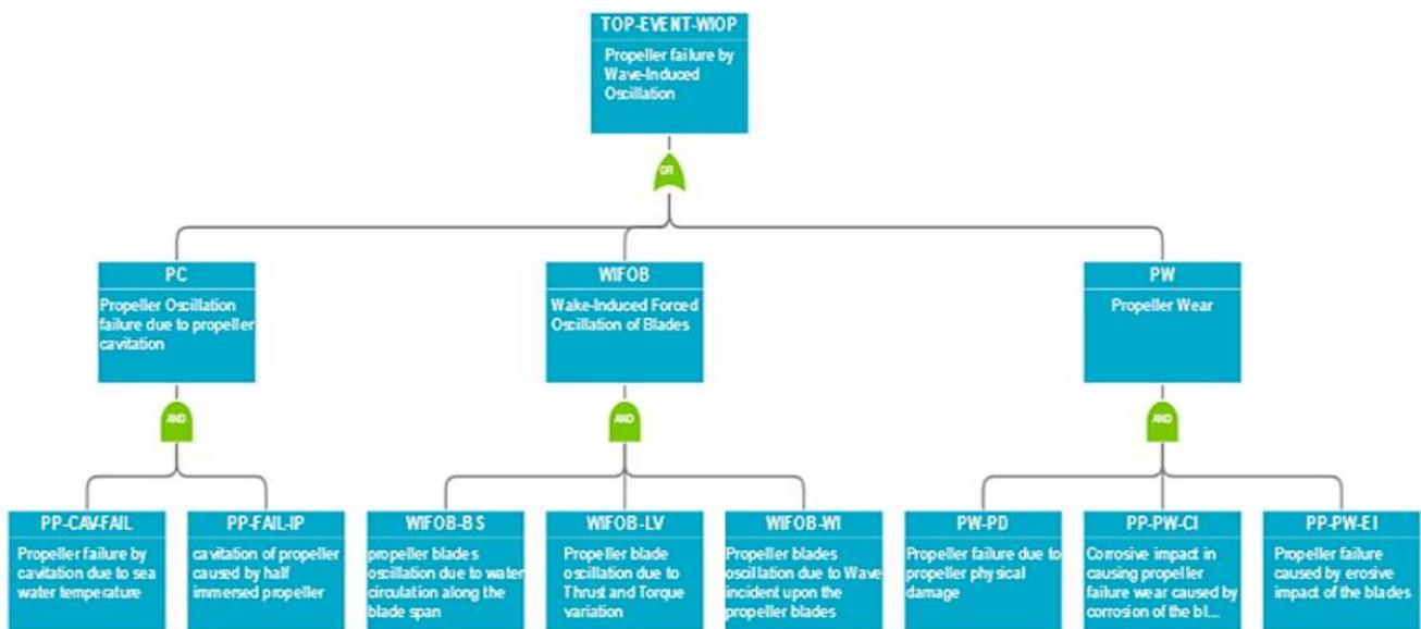
Figure 4. Fault tree analysis of propeller failure
