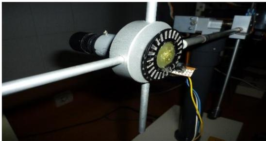
Figure 6. External incremental encoder & Optocoupler
