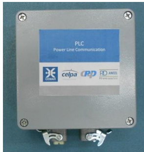
Figure 9. PLC transceiver in its enclosure.
