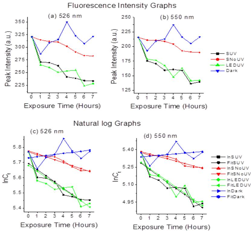
Figure 7. Variation of peak intensity with exposure time at 526 nm (a) and 550 nm (b) Natural log of fluorescence peak intensities at 526 nm (c) and 550 nm (d).
