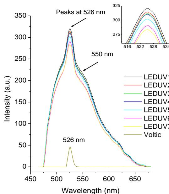
Figure 6. Variation in peak intensity with time of exposure for the water samples when exposed to the LEDUV radiation source.
