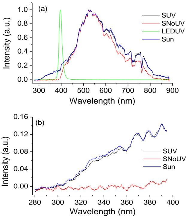
Figure 4. (a) Radiation sources SUV, SNoUV and LEDUV compared to sun's spectrum. (b) Comparison between SUV and SNoUV and sun's spectrum specifically within UV spectral regions. This shows transmitted and terminated wavelengths.
