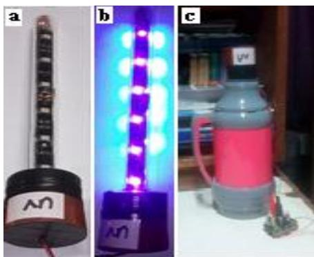
Figure 2. (a) LEDUV arranged on strips and wound round fabricated tube. (b) Powered LEDUV. (c) Purification chamber (flask) with the shielded LEDUV lowered into it
