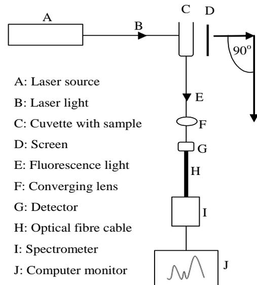
Figure 3. LIF setup for DOM measurements
