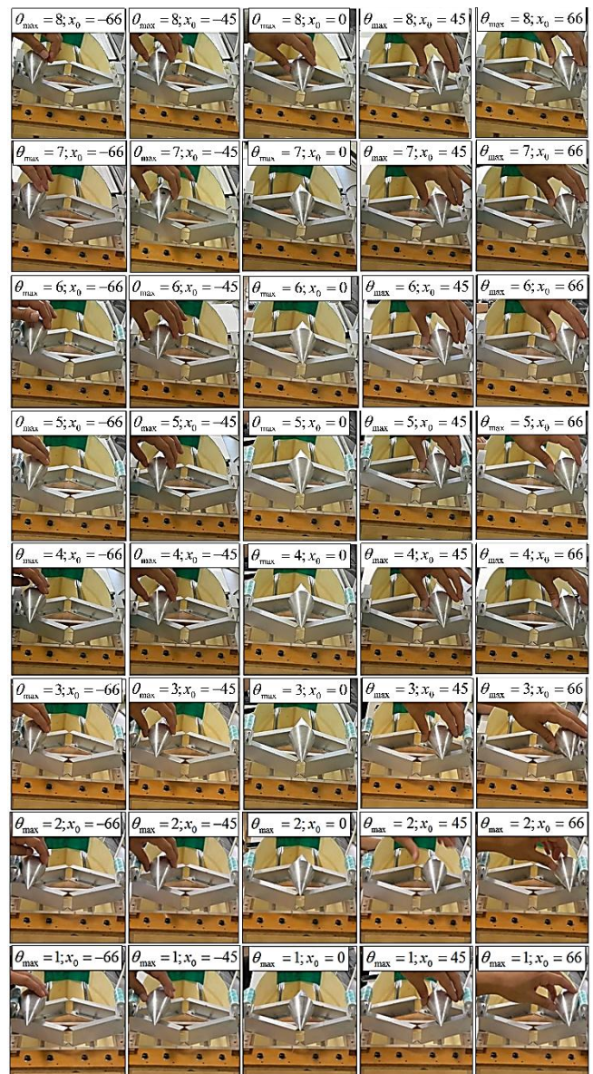
Figure 4. Snapshots of the double-cone, forcedly rolling on the divergent-convergent straight rails fixed at the ship hull, for different values of the maximal inclination angle and start coordinate.
