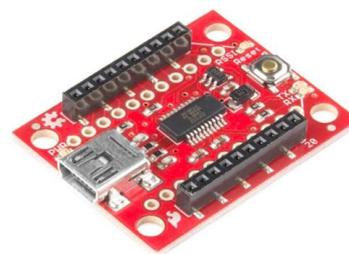
Figure 18. XBee Explorer
