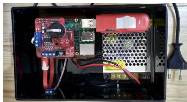
Figure 20. Remote Data Logger Hardware Platform
