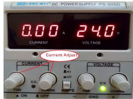
Figure 14. DC Current Source using Long Wei PS-305D
