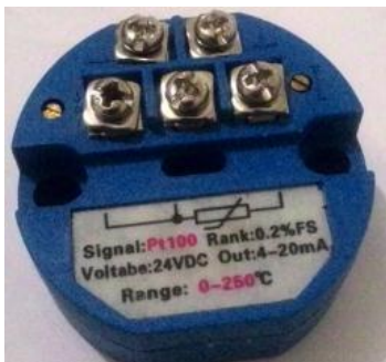
Figure 22. Transmitter PT100 4-20mA with Range 0-250°C
