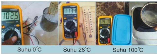
Figure 24. PT100 Sensor Test
