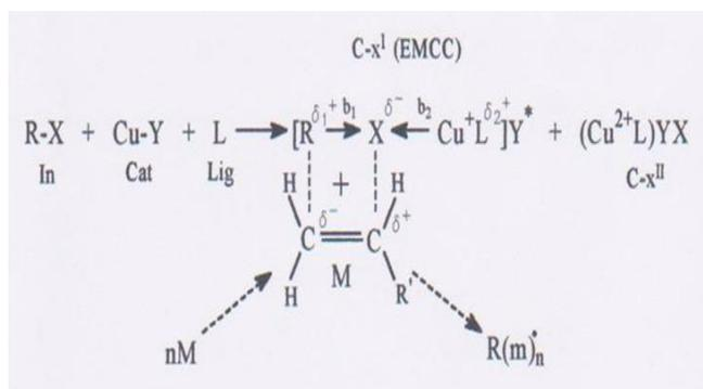
Figure 2. Scheme of two-centered electrostatic coordination of a monomer molecule (M) to an excited monovalent copper CT complex (C-xI; EMCC). In - initiator, Cat - catalyst, Lig - ligand, C-xII - bivalent copper complex.  $nM$  -  $n$  number of monomer molecules.  $R(m)_n$  - growing macroradical
