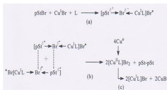
Figure 4. Scheme of bimolecular chain growth in ATRC, according to the PDFM theory. (a) formation of excited pSt complexes before the onset of the coupling reaction. (b) two-centered electrostatic coordination between pSt complexes, formation of pSt dimer in the coupling reaction, bimolecular completion of the chain growth, respectively. (c) deactivator reduction to its initial components by means of nanodispersed copper.
