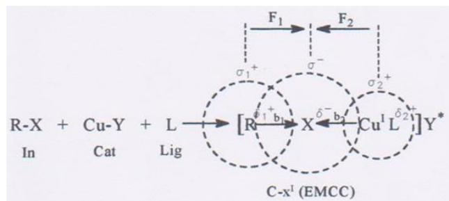
Figure 1. Scheme of excited monovalent copper CT formation according to the PDFM theory. In - initiator. Cat - catalyst. Lig - ligand. C-XI (EMCC) – excited monovalent copper complex. -X $\delta^-$  - central atom.  $b_1, b_2$  – semipolar bonds -  $\delta_1^+, \delta_2^+$  - electrostatic charges. -,  $\sigma_1^+, \sigma_2^+$  - superficial electrical densities.  $F_1, F_2$  – Coulomb forces.
