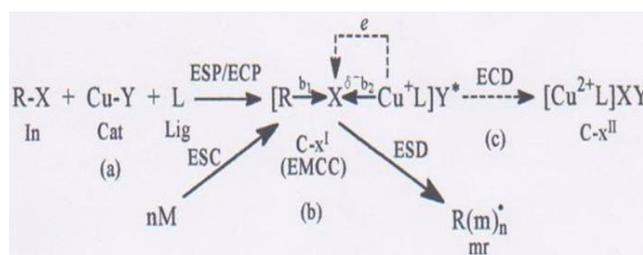
Figure 5. Generalized ATRP functional scheme. In – initiator. Cat – catalyst. Lig – ligand. C-xI (EMCC) – excited  $Cu^+$  complex. nM – n in number monomer molecules. ESC – two-centered electrostatic coordination process. ESP/ECP – electrostatic and electromechanical polarization of EMCC. ESD – electrostatic depolarization. ECD – electrochemical depolarization. mr – macroradical. e – electron. C-xII – inactive  $Cu^{2+}$  complex.
