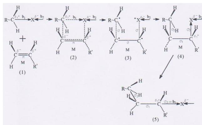
Figure 3. Scheme of two-centered electrostatic coordination and joining of a monomer molecule (M) to polar centers  $-C^{\delta^+} \rightarrow -X^{\delta^-}$ . Initial interaction, and subsequently, at each elementary act of monomolecular chain growth.  $\delta^-$  and  $\delta^+$  - partial electrostatic charges on carbon atoms of the monomer molecule.
