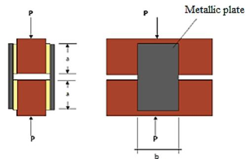
Figure 7. Shear Test – MR-14, RILEM (1993)
