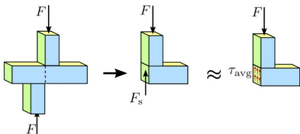
Figure 2. Shear stress in a horizontal bar loaded by two offset blocks, Sanpaz (2009)
