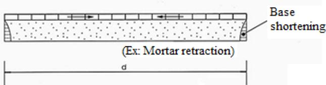
Figure 4. Ceramic coating required by compressive stress, Fiorito (2013)
