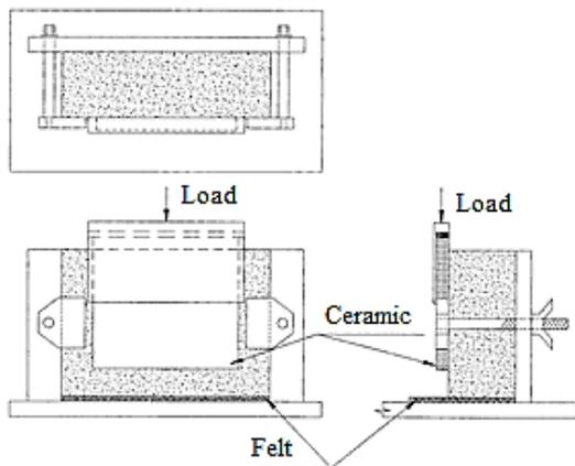
Figure 6. Test Method for Bond Strength of Ceramic Tile to Portland Cement Paste – ASTM C482, ASTM (2014)
