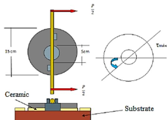
Figure 8. Torsion Test – MR-20, RILEM (1994)
