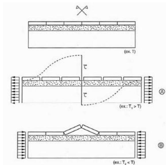
Figure 3. Ceramic coating required by tensile stress, Fiorito (2013)
