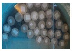
Figure 1. Submersible curing test specimens
