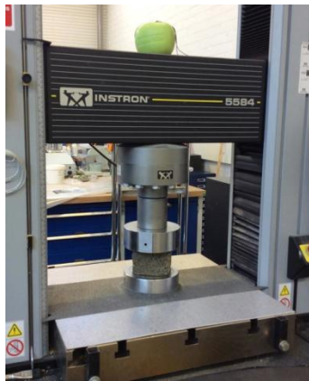
Figure 13. Equipment for Compressive Test
