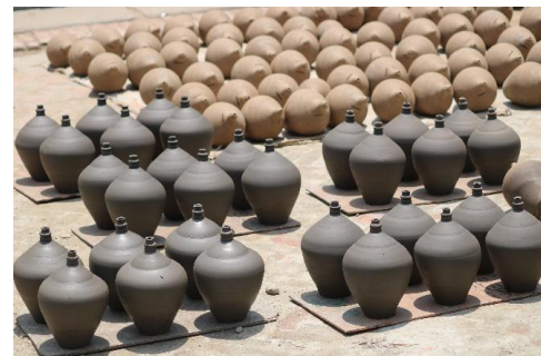
Figure 2. Drying of the Piggy Bank
