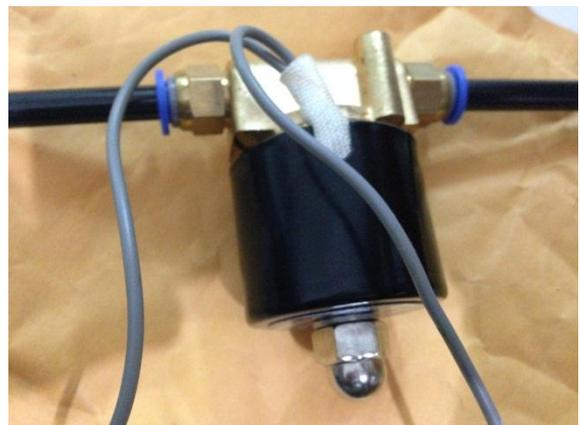
Figure 7. Automated on/off valve
