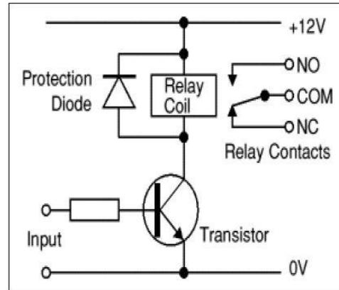
Figure 6. Relay Circuit
