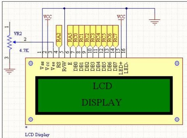
Figure 8. LCD Display Schematic Diagram
