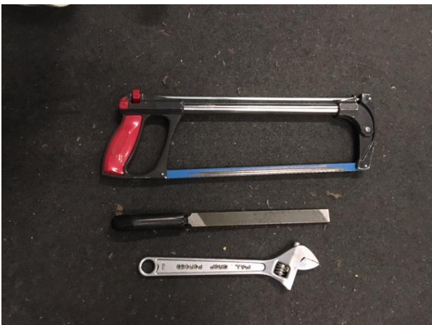
Figure 2. Retrofitting tools: hacksaw, file and crescent wrench
