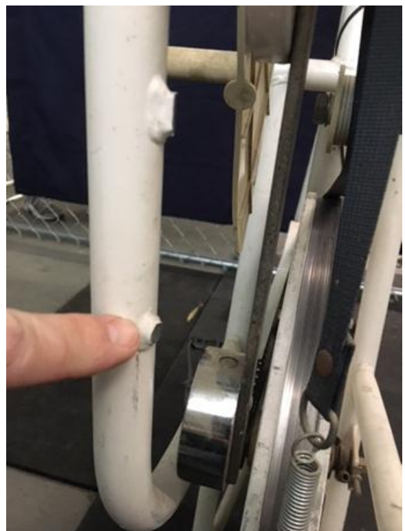
Figure 5. Front view of pendulum stop removed
