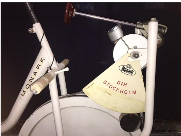
Figure 3. Close-up of the pendulum assembly
