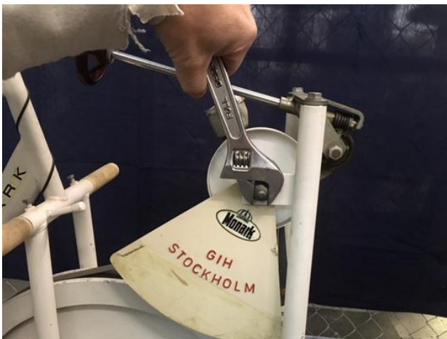
Figure 6. Loosen bolt to shift pendulum reader
