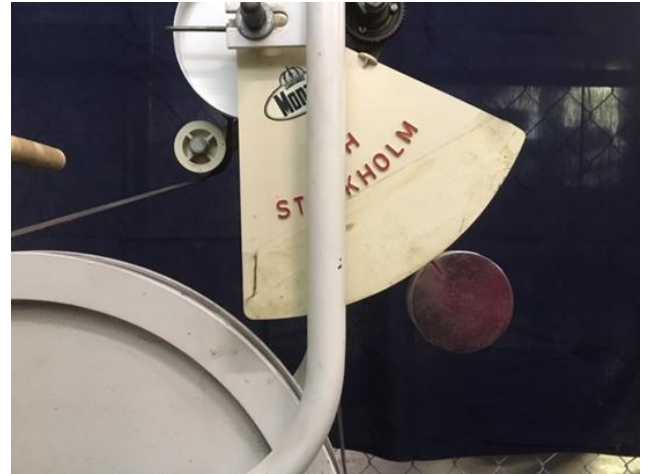
Figure 8. Pedaling backwards will cause the pendulum to swing forward where by the load can be assessed by viewing the pendulum reader
