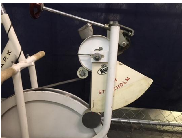
Figure 7. Pendulum positioned to allow backward pedaling
