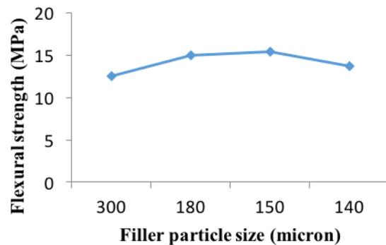
Figure 2. The effect of particle size of filler on flexural strength of wasted Styrofoam filled with sawdust
