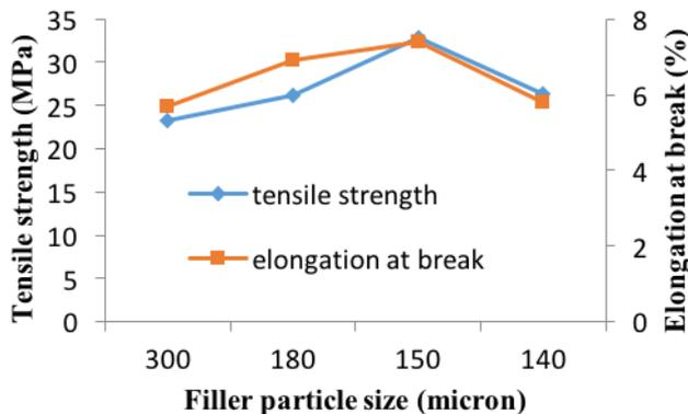
Figure 1. The effect of particle size of filler on tensile strength and elongation at break of Styrofoam filled with sawdust composites
