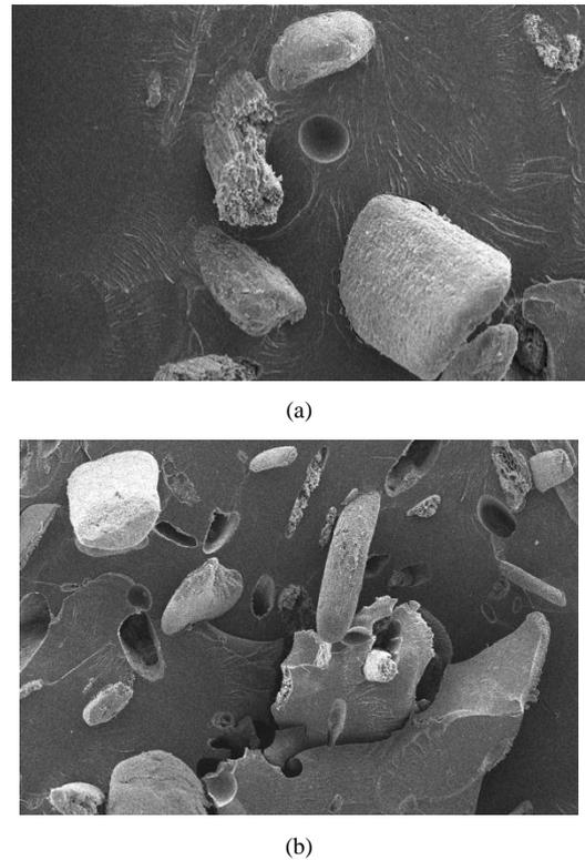
Figure 4. SEM micrographs of surface Styrofoam-sawdust composite: (a) 150 micron; (b) 140 micron
