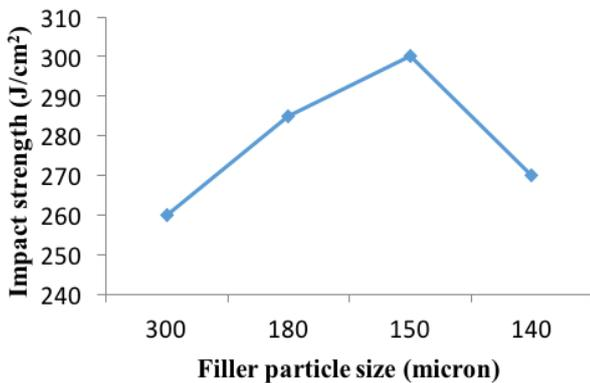
Figure 3. The effect of particle size on the impact strength of wasted Styrofoam filled with sawdust.
