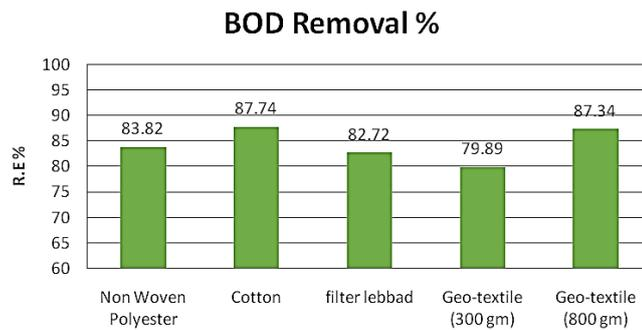
Figure 7. BOD Removal efficiency of Gravity filter
