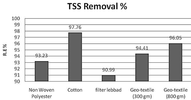
Figure 6. TSS Removal efficiency of Gravity filter
