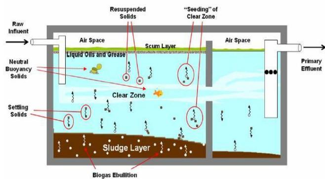
Figure 2. Septic tank processes
