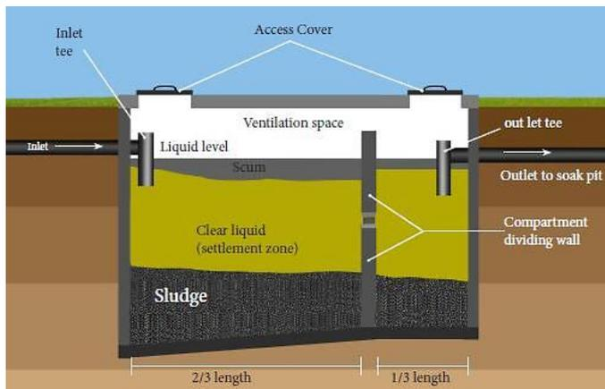
Figure 1. Typical septic tank
