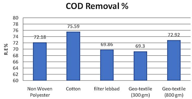
Figure 8. COD Removal efficiency of Gravity filter
