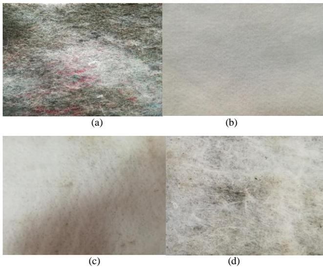
Figure 3. Examined materials (a) Filter labbad (b) Non-woven geo-textile 300 gm (c) Non-woven geo-textile 800 gm (d) Non-woven polyester
