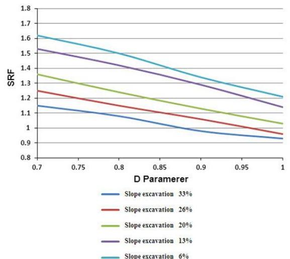
Figure 9. The SRF variations with different excavation percentages according to the D parameter in the slope of 60 degree.
