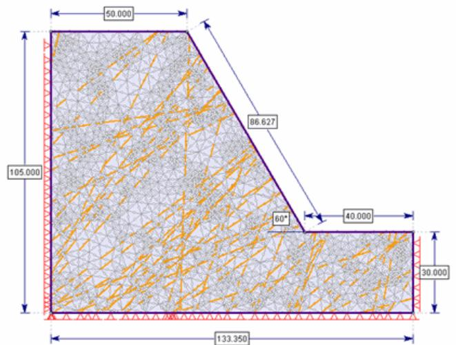
Figure 2. The modeled slope with dip of 60 degree
