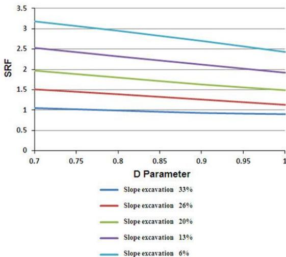
Figure 7. The SRF variations with different excavation percentages according to the D parameter in the slope of 30 degree.
