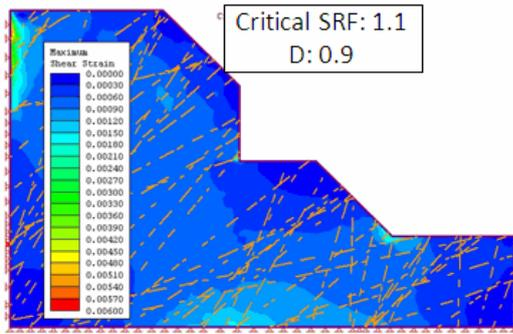
Figure 5. The critical SRF for slope with dip of 45 degree and 33% excavation (D parameter is 0.9)
