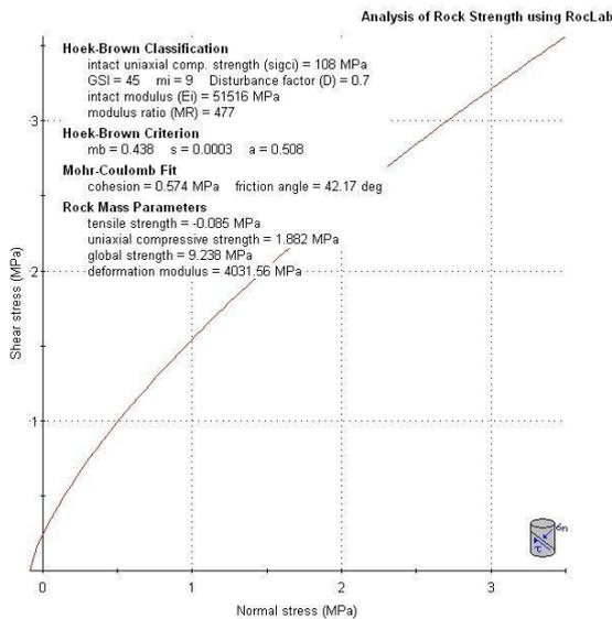
Figure 1. The geomechanical parameters of dolomitic rock masses
