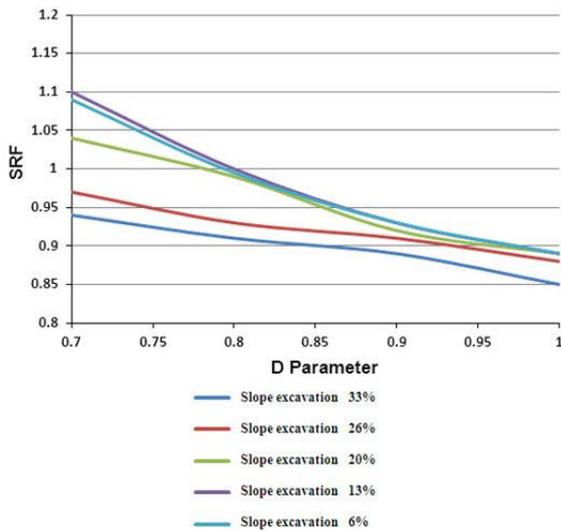
Figure 10. The SRF variations with different excavation percentages according to the D parameter in the slope of 75 degree.
