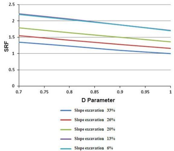
Figure 8. The SRF variations with different excavation percentages according to the D parameter in the slope of 45 degree.
