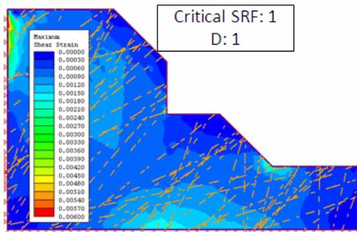
Figure 6. The critical SRF for slope with dip of 45 degree and 33% excavation (D parameter is 1)
