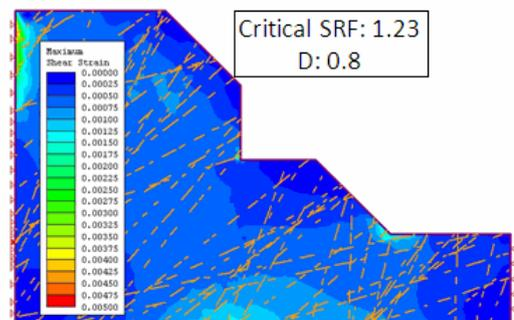
Figure 4. The critical SRF for slope with dip of 45 degree and 33% excavation (D parameter is 0.8)
