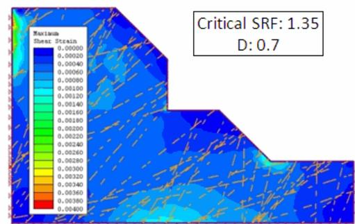
Figure 3. The critical SRF for slope with dip of 45 degree and 33% excavation (D parameter is 0.7)
