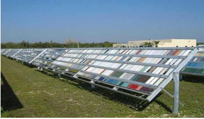
Figure 1. Specimens aging on 45° test racks. <www.q-lab.com>
