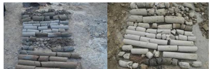
Figure 1. Core samples of soil-cement mixtures
