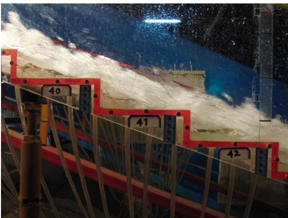
Figure 5. Nappe flow regime in Discharge 20 liters per second and flat steps
