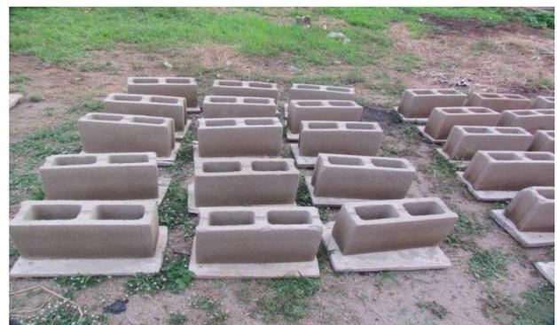
Figure 3. Blocks produced from 98% sand and 2% sawdust
