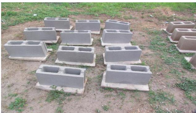
Figure 2. Blocks produced from 100% sand and 0% sawdust replacement
