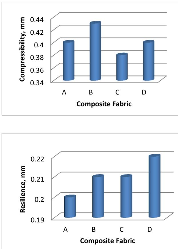
Figure 8. Compressibility and resilience properties of composite fabrics
