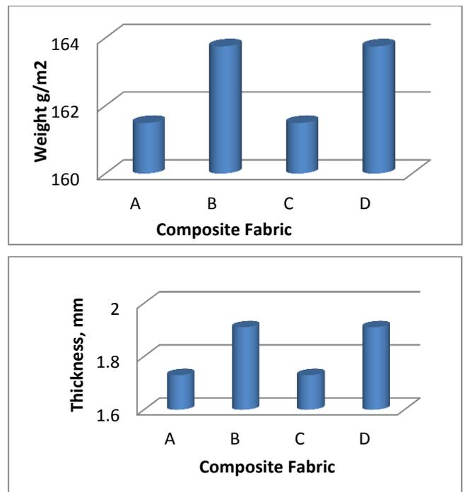
Figure 4. Weight and thickness of composite fabrics
