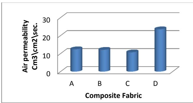
Figure 5. Air permeability of composite fabrics
