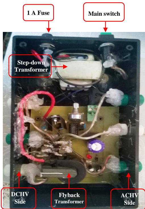
Figure 11. A PCB circuit printed inside box
