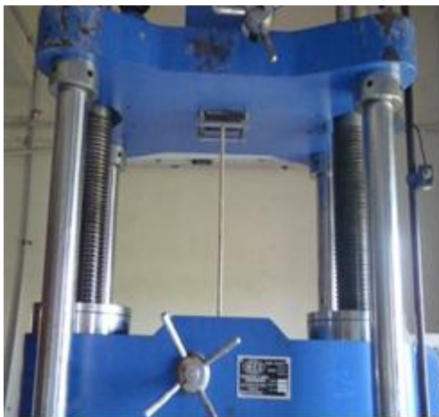
Figure 3. GFRP Reinforcement under Tension Test
