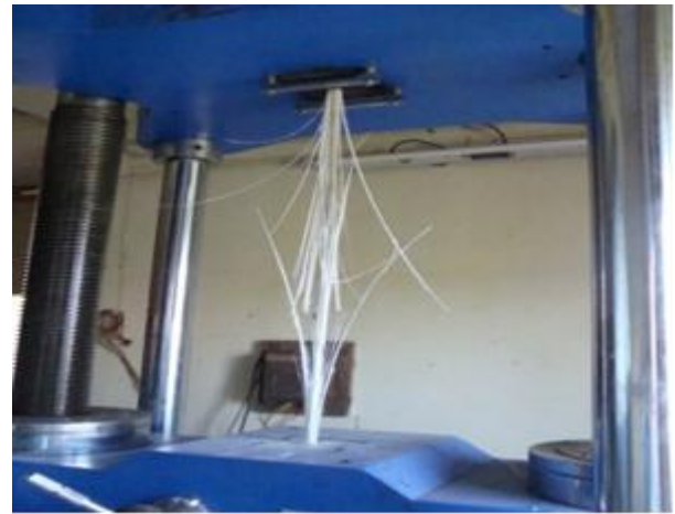
Figure 4. Tensile Failure Mode of GFRP Reinforcement
