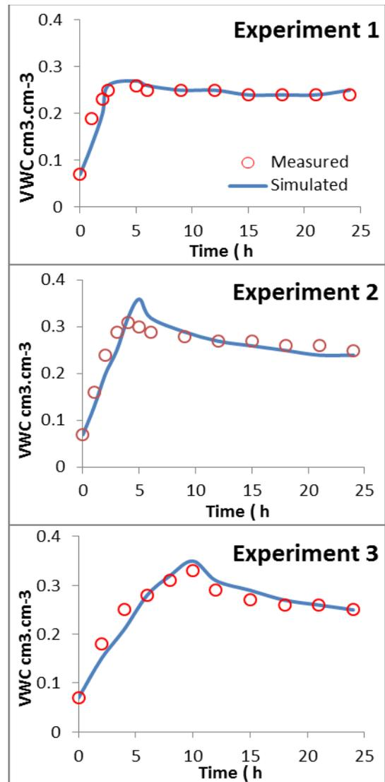
Figure 4. The comparison between the rate of volumetric water content measured in the field and simulated by program Hydrus 2D for experience 1, 2 and 3, for all depths and 24 h from the start of the irrigation period
