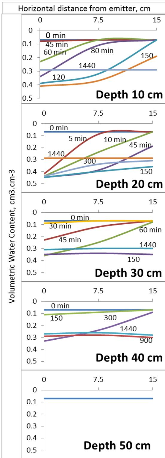
Figure 1. Distribution and redistribution of water for experiment 1 (irrigation period 2.5 h) during 24 hours from the start of irrigation
