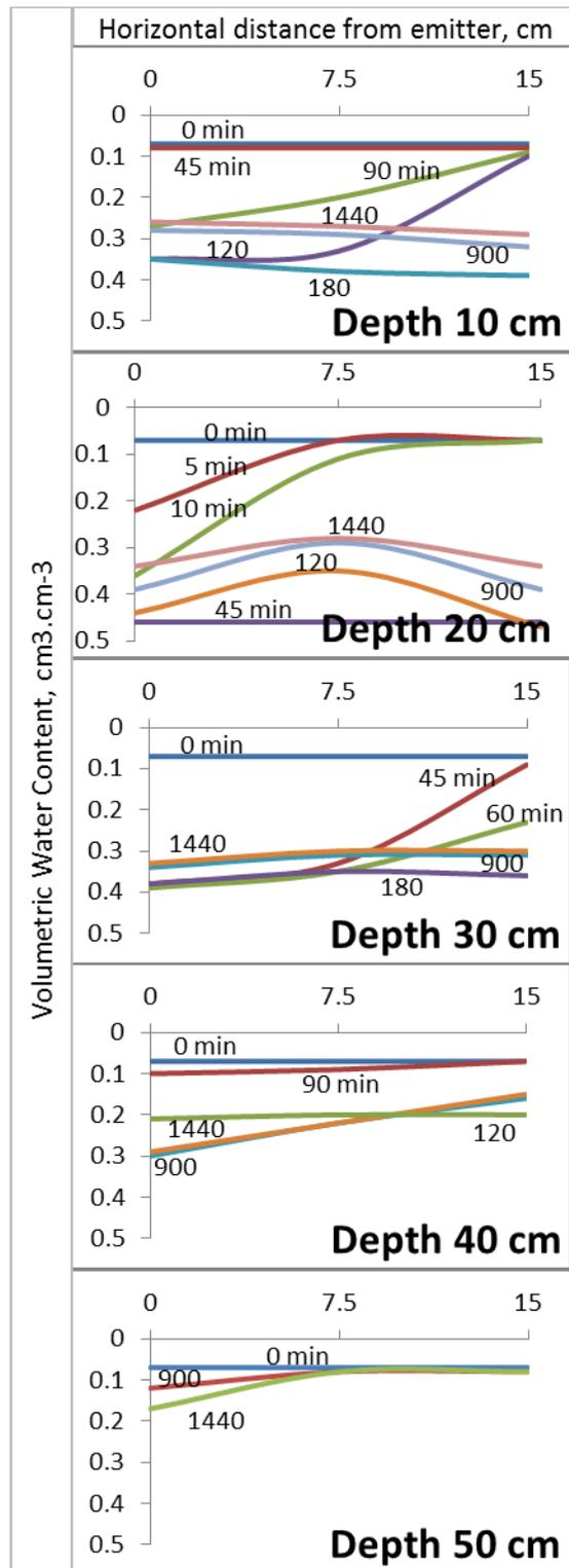
Figure 2. Distribution and redistribution of water for experiment 2 (irrigation period 5.0 h) during 24 hours from the start of irrigation
