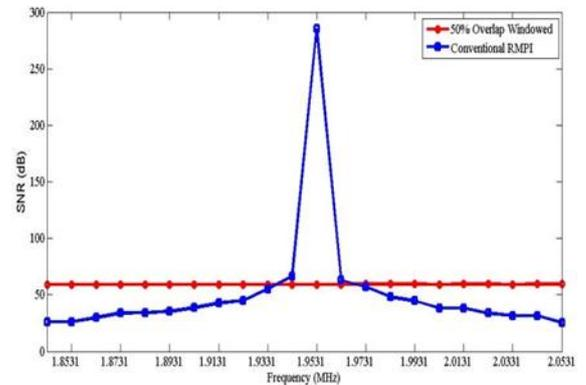
Figure 4. Comparison of recovery of a conventional RMPI and the proposed architecture
