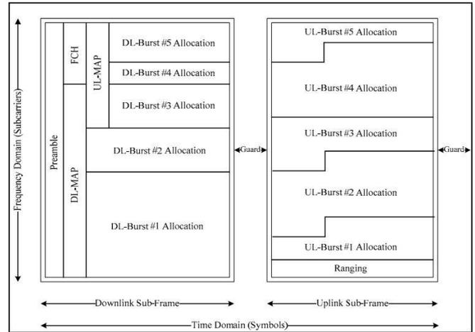
Figure 1. Wimax TDD Frame structure
