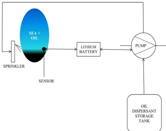
Figure 2. Block diagram of the Automatic Oil Spill Dispeller
