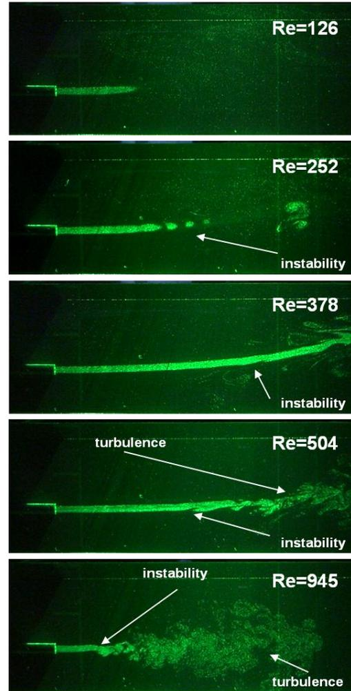
Figure 3. Laminar to Turbulent Transition of a Submerge Jet Flow
