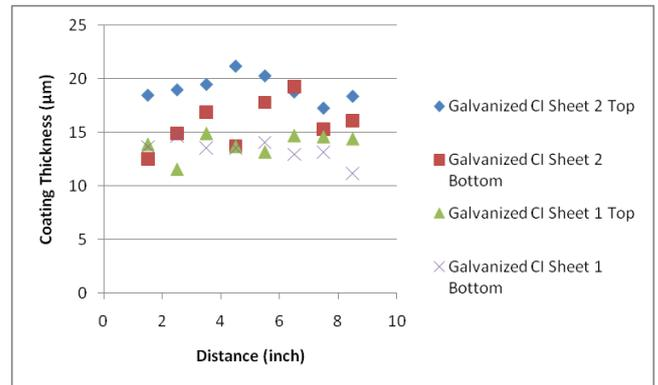
Figure 1. Comparison between the thicknesses of two galvanized CI sheets.
