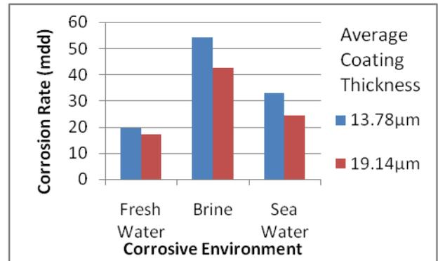
Figure 4. Effect of Coating Thickness on the Corrosion rate of galvanized CI sheets after being exposed in three different environments for 70 hours.
