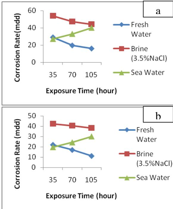
Figure 2. Corrosion rate with exposure time in three different environments. (a) Galvanized CI sheet 1 (b) Galvanized CI sheet 2.
