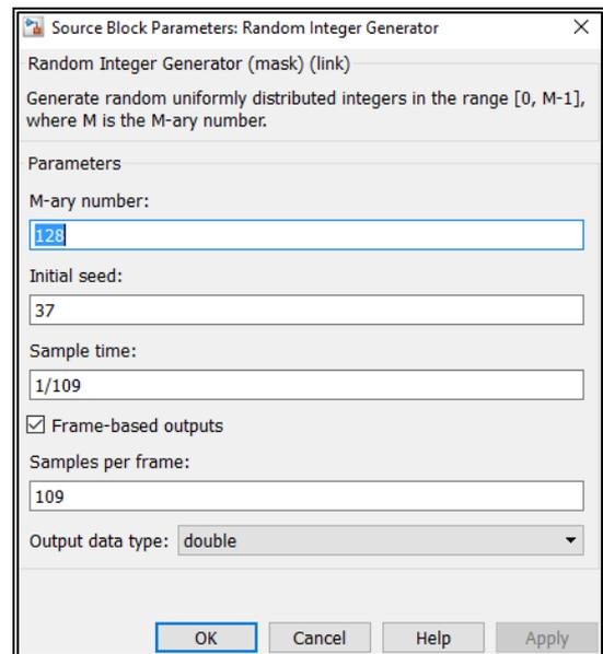
Figure 1. Configuration parameters for the Random integer generator
