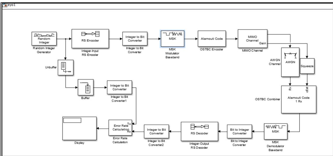
Figure 8. Simulink model for 2X1 MIMO-MSK system with RS code in a noisy multipath Rayleigh channel
