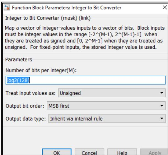
Figure 3. Configuration parameters for the Bit to Integer, and Integer to Bit blocks
