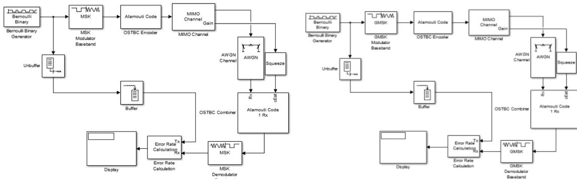
Figure 9. Simulink model for 2X1 MIMO-MSK & MIMO-GMSK without RS code in a noisy multipath Rayleigh channel
