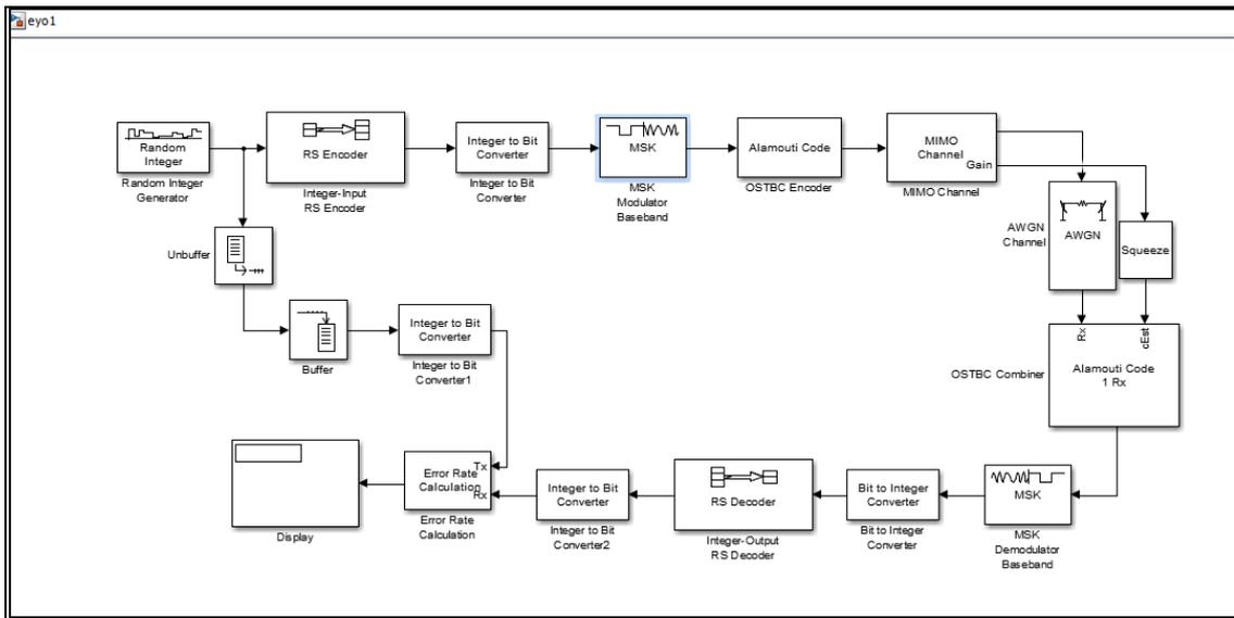
Figure 7. Simulink model for 2X1 MIMO-GMSK system with RS code in a noisy multipath Rayleigh channel
