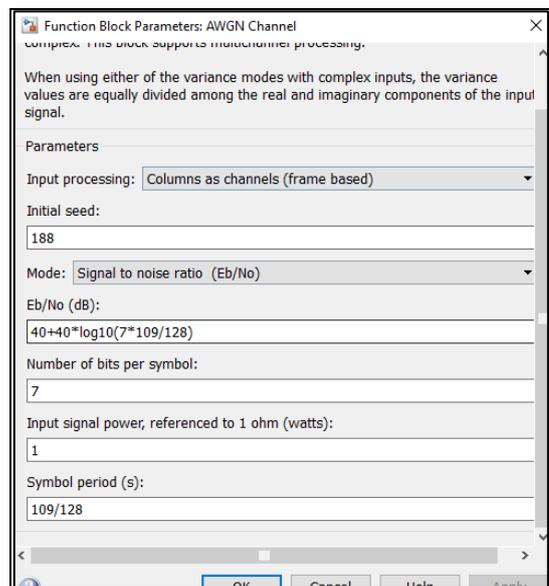
Figure 6. Configuration parameters for the AWGN block
