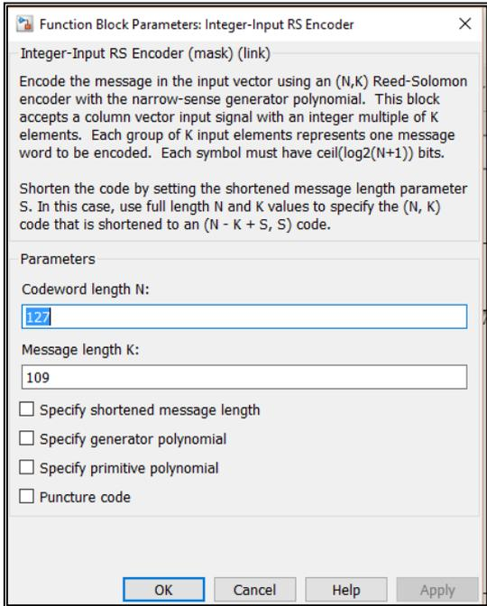
Figure 2. Configuration Parameters for the Integer-input RS encoder & Integer-output RS decoder
