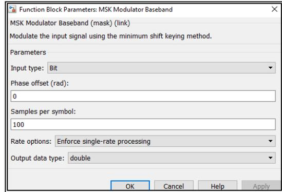
Figure 4. Configuration parameters for the GMSK & MSK modulator baseband blocks
