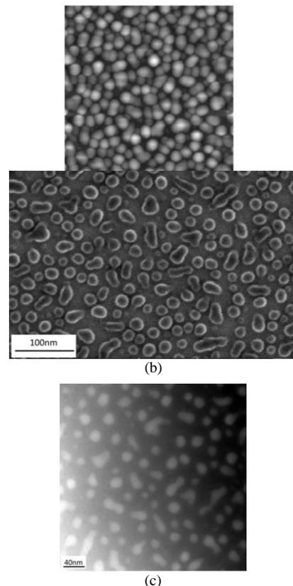
Figure 1. Si nanoparticle images obtained by (a) AFM, (b) SEM and (c) TEM.
