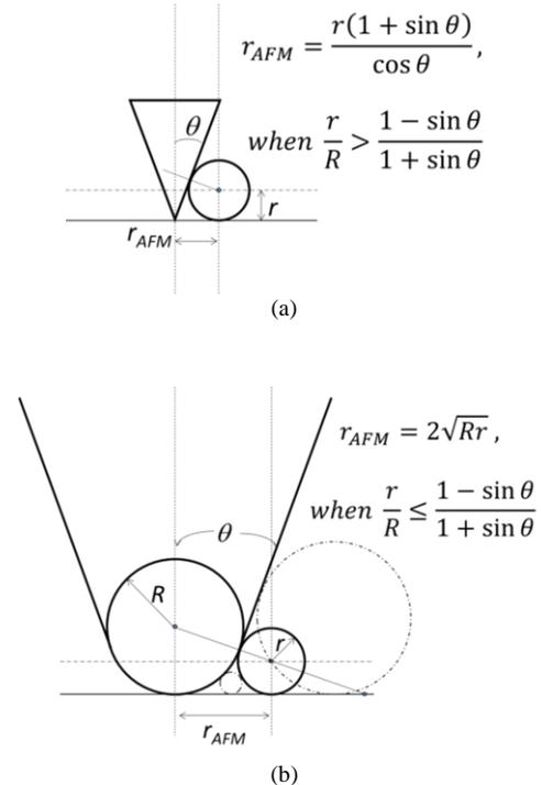
Figure 3. Relationship of AFM tip's geometry  $\theta$ , actual particle size  $r$  and the measured particle size  $r_{AFM}$ .
