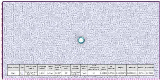
Figure 2. The modeling of circular tunnel with diameter of 8 meters and at a depth of 50 meters that reinforced with lining
