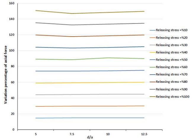
Figure 9. The diagram shows the effect of releasing stress in the new tunnel on the axial force of lining in the old tunnel at a depth of 50 meters ( $d$ =tunnels distance;  $a$ =tunnel radius)
