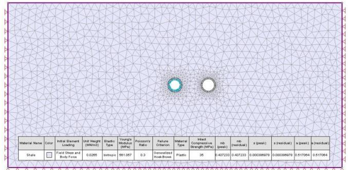
Figure 4. The modeling of a circular tunnel (new tunnel) with diameter of 8 meters at a distance of 20 meters from the previous tunnel
