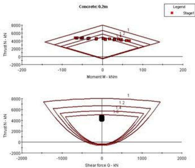
Figure 12. Support capacity diagrams for tunnel lining (releasing stress in adjacent tunnel is equal to 100 percent)
