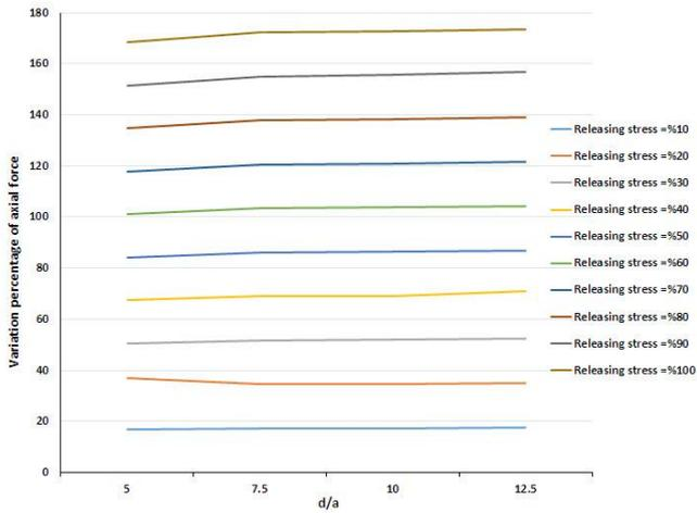
Figure 6. The diagram shows the effect of releasing stress in the new tunnel on the axial force of lining in the old tunnel at a depth of 20 meters ( $d$ =tunnels distance;  $a$ =tunnel radius)
