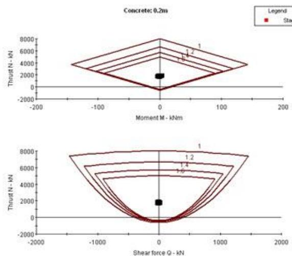
Figure 10. Support capacity diagrams for tunnel lining (releasing stress in adjacent tunnel is equal to 10 percent)
