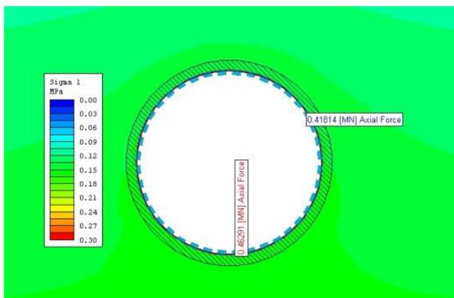
Figure 3. The values of axial force in the lining of circular tunnel with diameter of 8 meters and at a depth of 50 meters
