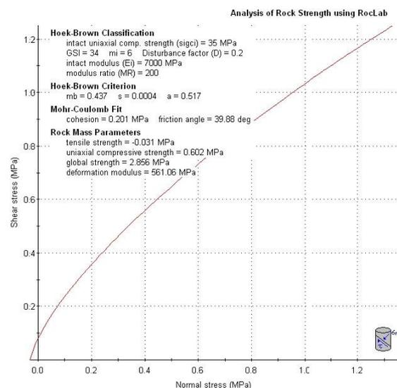
Figure 1. The geomechanical parameters of shale rock masses
