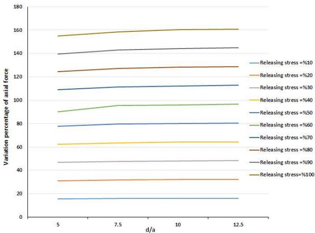
Figure 7. The diagram shows the effect of releasing stress in the new tunnel on the axial force of lining in the old tunnel at a depth of 30 meters ( $d$ =tunnels distance;  $a$ =tunnel radius)
