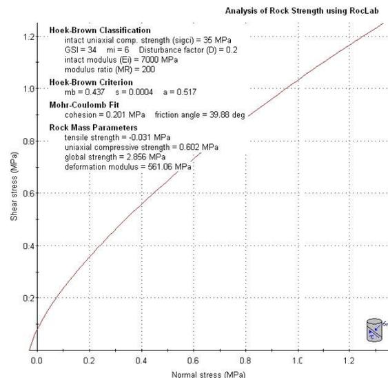
Figure 1. The geomechanical parameters of shale rock masses
