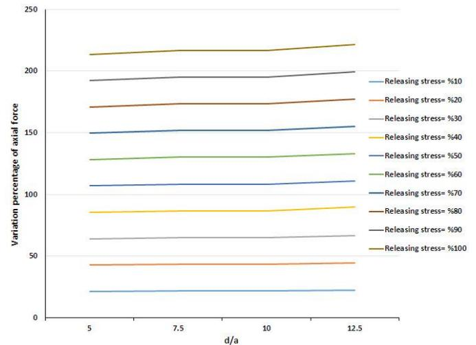
Figure 5. The diagram shows the effect of releasing stress in the new tunnel on the axial force of lining in the old tunnel at a depth of 10 meters ( $d$ =tunnels distance;  $a$ =tunnel radius)
