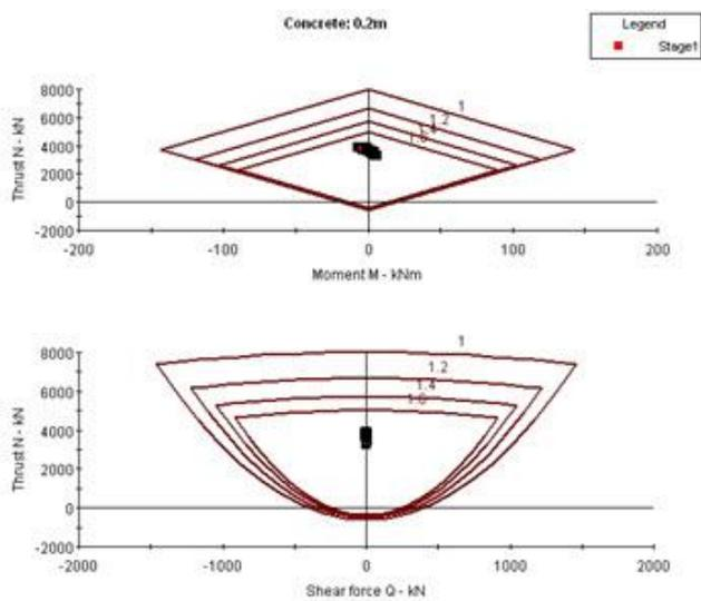
Figure 11. Support capacity diagrams for tunnel lining (releasing stress in adjacent tunnel is equal to 50 percent)
