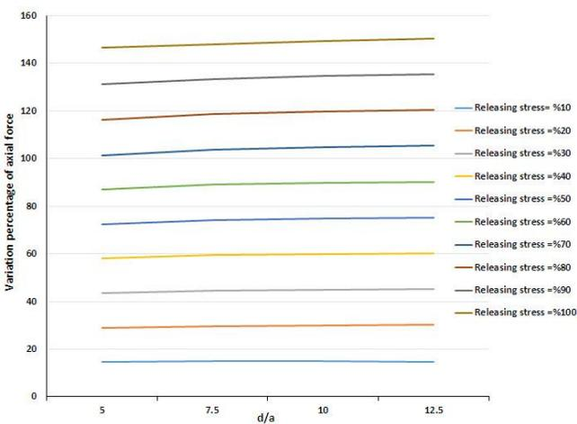
Figure 8. The diagram shows the effect of releasing stress in the new tunnel on the axial force of lining in the old tunnel at a depth of 40 meters ( $d$ =tunnels distance;  $a$ =tunnel radius)
