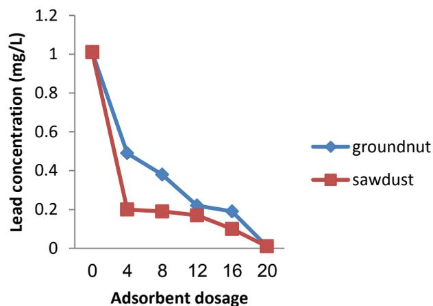
Figure 4. Variation of lead concentration with varying dosages of different adsorbates.
