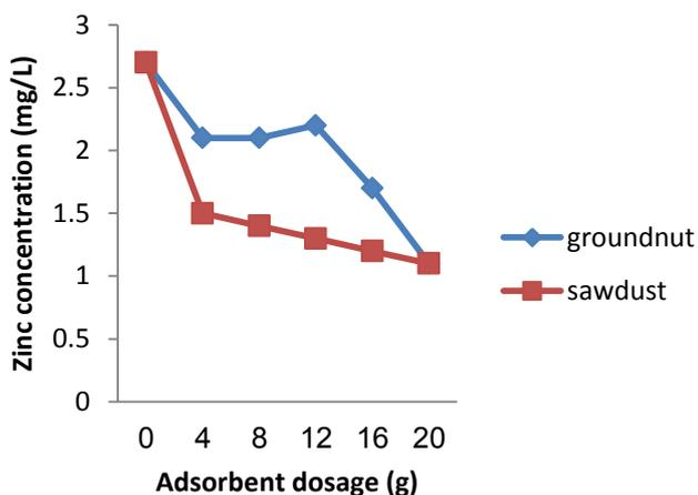
Figure 1. Variation of zinc concentration with varying dosages of different adsorbates.
