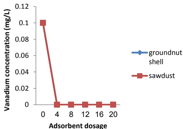
Figure 5. Variation of vanadium concentration with varying dosages of different adsorbates.
