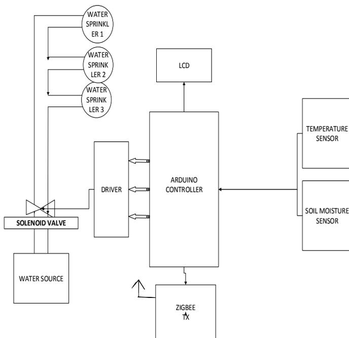
Figure 1. Block Diagram of the System Transmitter
