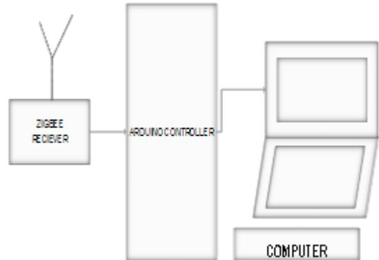
Figure 6. Block Diagram of the System Receiver
