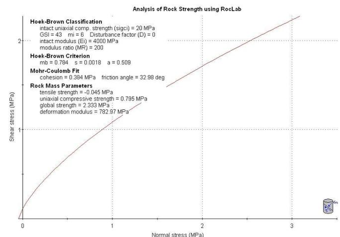
Figure 1. The geomechanical parameters of shale rock masses
