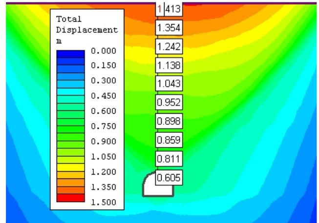
Figure 3. Displacements in the tunnel roof in deterministic analysis
