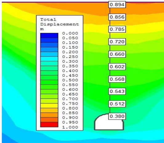
Figure 5. Displacements in the tunnel roof in probabilistic stability analysis (the standard deviation to 3 for deformation modulus)
