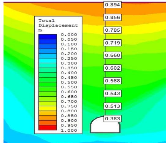
Figure 7. Displacements in the tunnel roof in probabilistic stability analysis (the standard deviation to 3 for intact uniaxial compressive strength)
