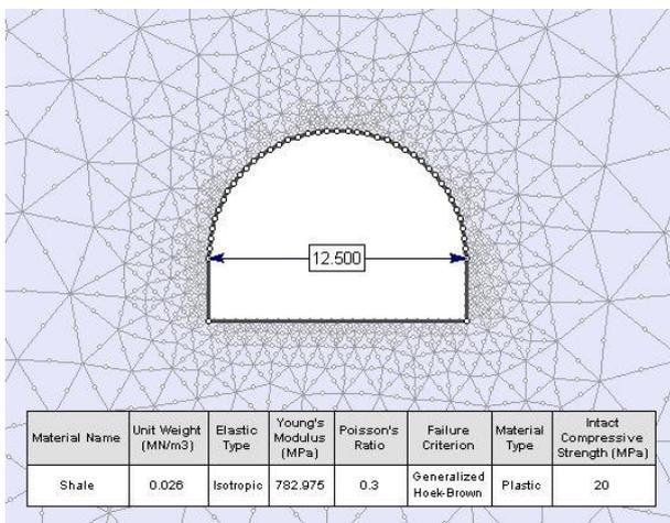
Figure 2. Numerical modeling of the tunnel No.2 of Kurdistan
