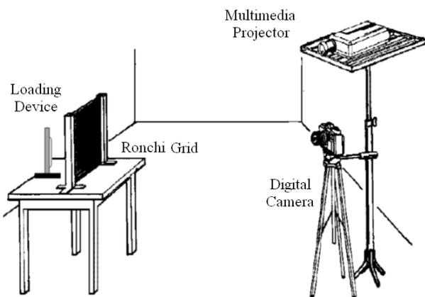
Figure 1. Experimental setup for shadow *moiré*. Hertz et al., 1.995
