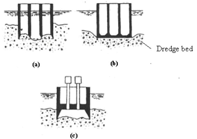
Figure 9. Various types of caisson foundations; a) open, b) box ,c) pneumatic
