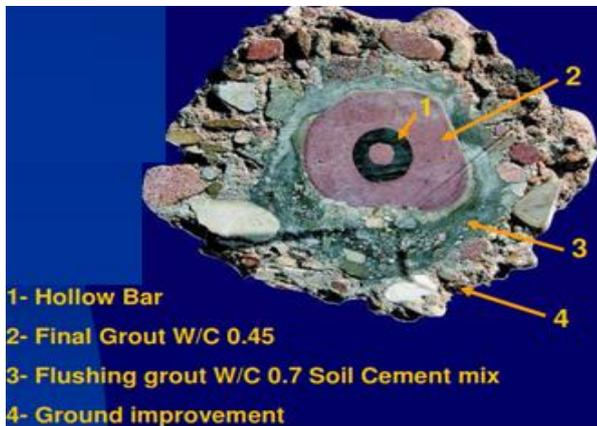
Figure 11. Typical cross section of an exhumed micro pile [7]
