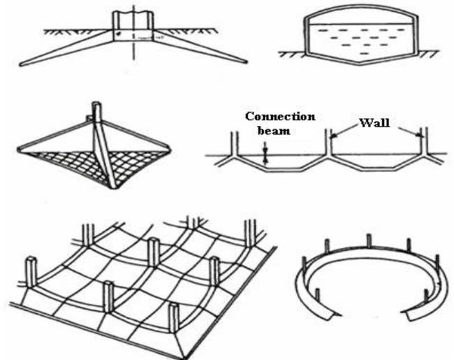
Figure 13. Examples of shell foundations
