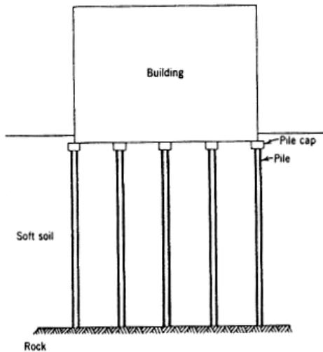
Figure 5. Building with pile foundation [4]
