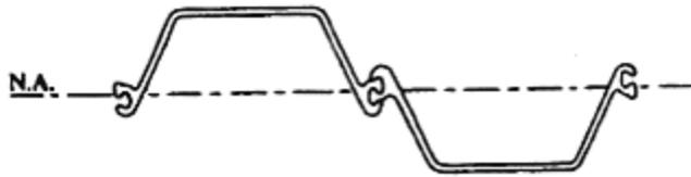
Figure 14. Cross section for one type of sheet pile connection
