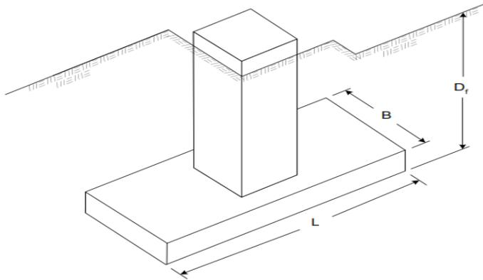
Figure 1. Rectangular single footing [1]  $D_f$  (depth of footing),  $B$  (width of footing),  $L$  (length of footing)
