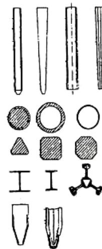
Figure 7. Profiles / cross sections used for driven piles
